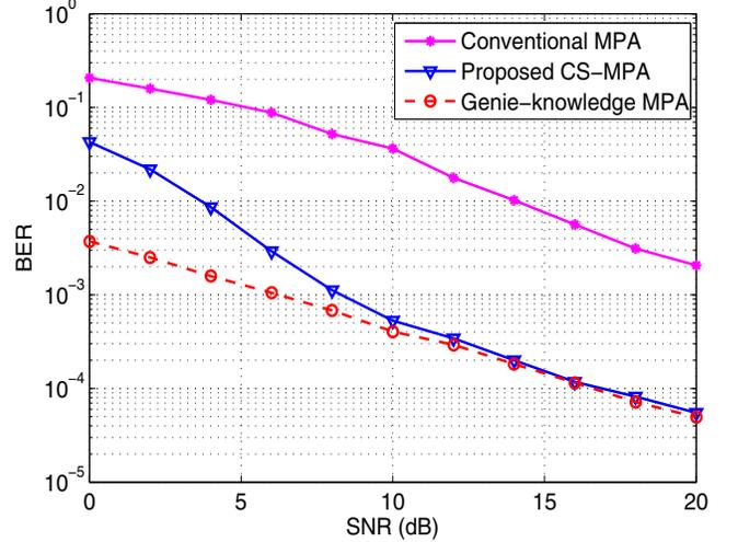
Fig. 4. BER performance of the proposed CS-MPA detector.
