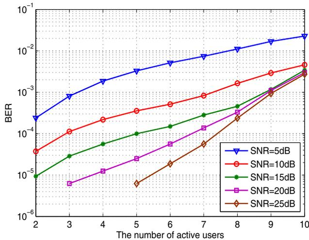
Fig. 5. BER performance of the proposed CS-MPA detector.
