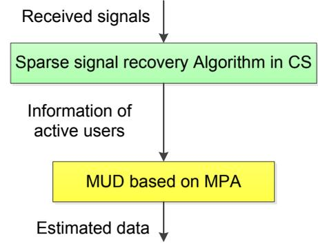
Fig. 3. Diagram representation of the proposed CS-MPA detector.
