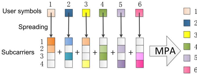
Fig. 1. Graphical representation of LDS-OFDM, where  $K = 6$  active users occupied  $N = 4$  subcarriers, leading to the overloading factor 150%.
